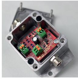
The electronics in the DMPE are housed in a robust metal casing that is dust and water-protected.
